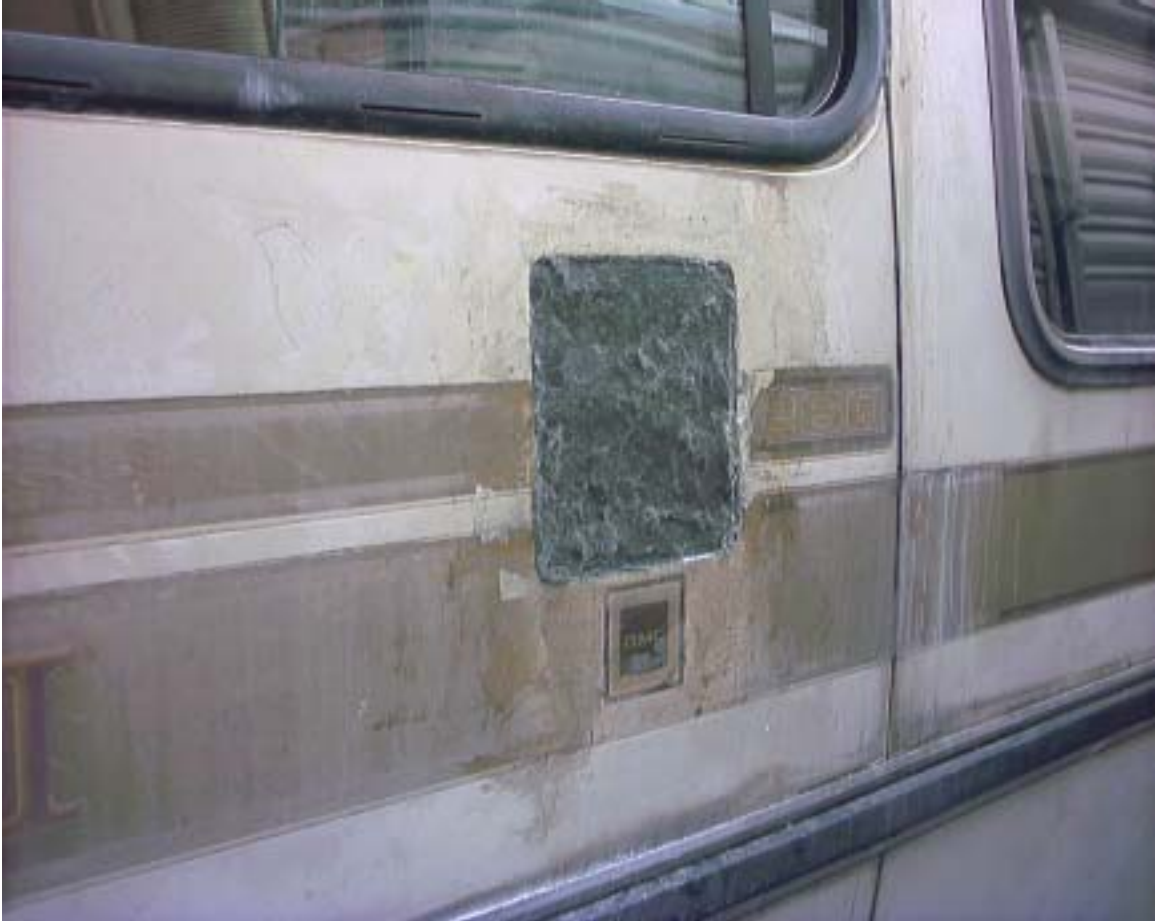
The “Dyna-Hair” forms a strong patch due to the fiberglass fibers suspended in the resin.
