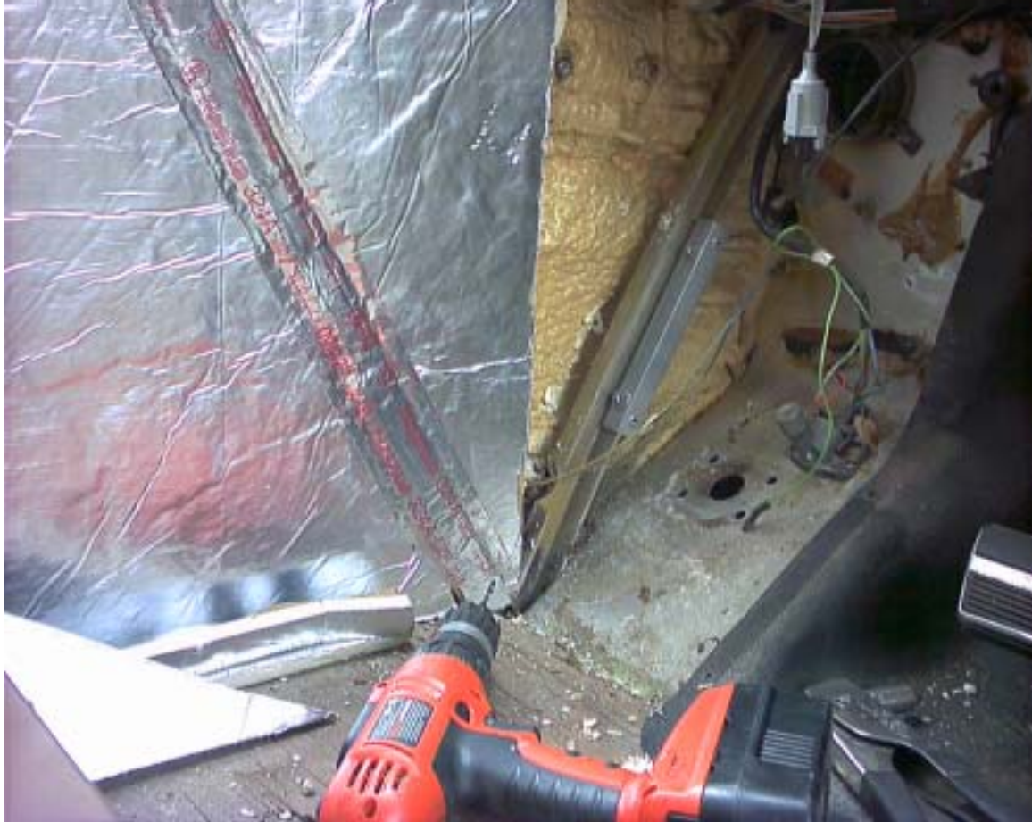
The Aluminum angle bracket provides a fastening point for the new FRP kick panel.
