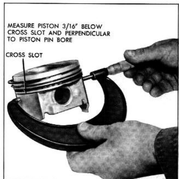
Fig. 6-143 Measuring Piston Diameter
